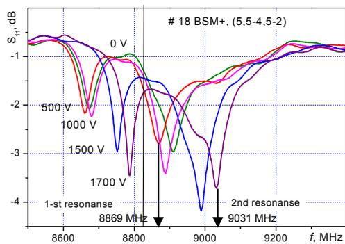
Figure 2: S11 parameters of the X band “transparent contact” resonator. BSM substrate  $23 \times 19 \times 1.0$  mm<sup>3</sup>, permittivity of the ceramic and ferroelectric of 20 and 481 respectively, frequency shift of 116 MHz (first resonance) and 162 MHz (second resonance) at a 1.7 V/ $\mu$ m bias field.
