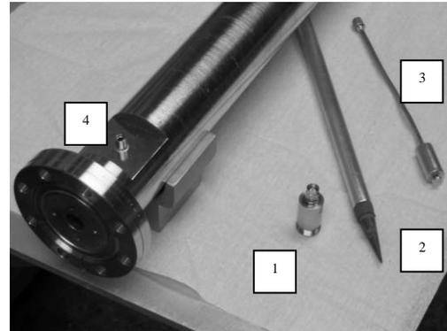
Figure 2. 13.625 GHz DLA structure for the ETR experiment with a probe for wakefield measurements (1); RF power absorber (2) and coupler (3) for bench testing; current probe feedthrough from the DLA structure (4).
