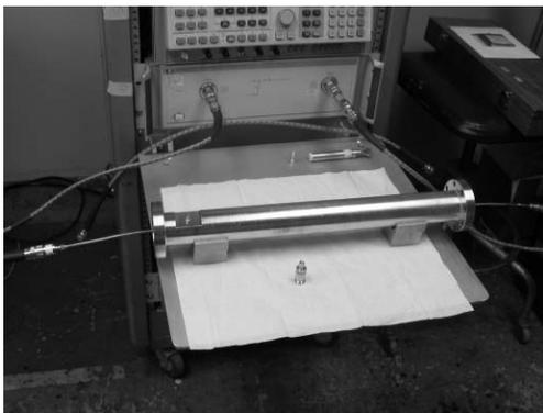
Figure 1. Bench test of the 13.625 GHz dielectric based accelerating structure at Argonne Wakefield Accelerator, Argonne National Laboratory.
