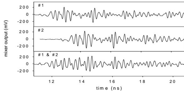
Figure 4. Experimental results using the new AWA gun and linac to excite a wakefield using a two bunch train. Each bunch has an intensity of 15 nC. #1 is the wakefields of beam 1 alone, #2 of the beam 2 alone, #3 wakefields of the two bunches simultaneously.
