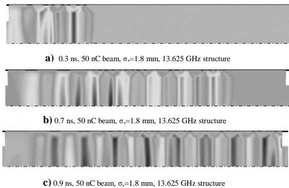
Figure 3. Single beam wakefields snapshots in the 13.625 GHz DLA structure. The beam charge is 50 nC, and bunch length is 1.8 mm. Snapshots at a) - 0.3 nsec, b) - 0.7 nsec and c) - 0.9 ns.
