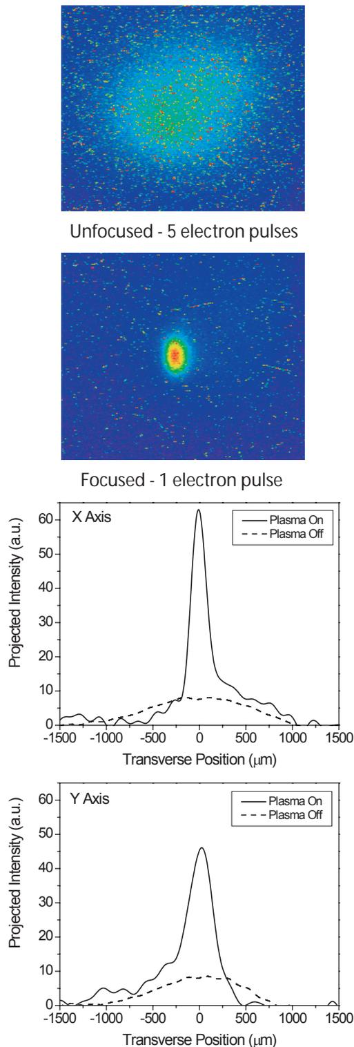
Figure 2: First Frame (Top): False color image of the unfocused electron beam spot, shown at five times normal intensity in order to provide sufficient image contrast, on the OTR screen after the plasma lens. Second Frame: False color image of the plasma focused electron beam spot on the OTR screen. Third and Fourth Frames: Plots of the image intensity of the above photographs (normalized to 1 electron pulse) in the x axis (third) and y axis (fourth).
