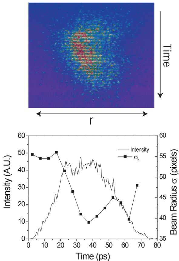
Figure 3: A false color streak camera image of the plasma focused beam (top) with initial analysis of the image (bottom).
