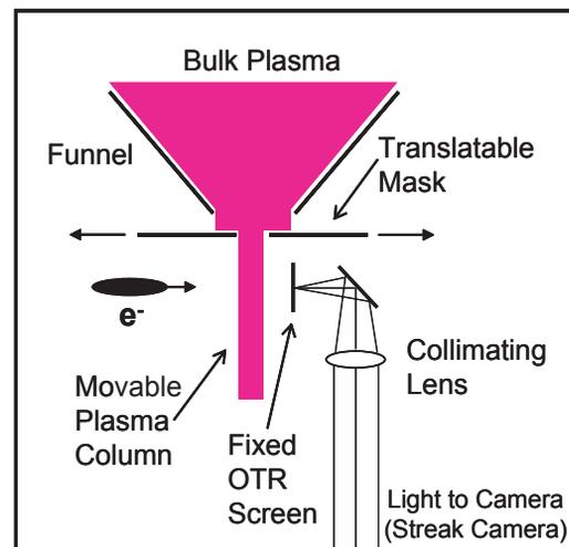
Figure 1: Schematic of the plasma lens apparatus.
