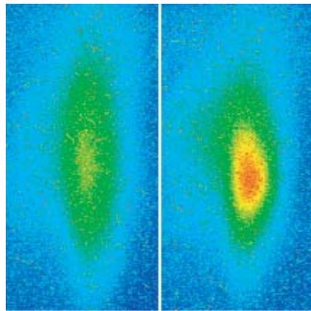
Figure 4: False color images of a beam with an initial 1:3.4 aspect ratio. At left the plasma is off, at right the plasma is on. Both images show the same number of beam pulses.
