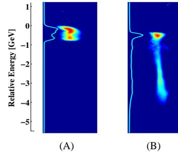
Figure 2: The images are plotted with a logarithmic color map in order to bring out the tails. (A)  $N = 0.61 \times 10^{10}$  and no ionization occurs. (B)  $N = 1.43 \times 10^{10}$  fully ionizes the Li vapor.
