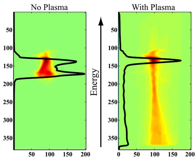
Figure 5: Spectrometer images of two shots, without and then with the plasma cell in the beam. The high energy nose cannot ionize lithium, so goes through unimpeded in both cases. Only later portions of the bunch experience the plasma effects with strong acceleration and deceleration. Vertical axis is pixels on spectrometer camera.
