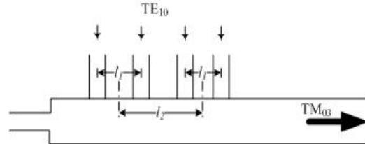
Figure 2: Schematic drawing of mode selective coupler.
