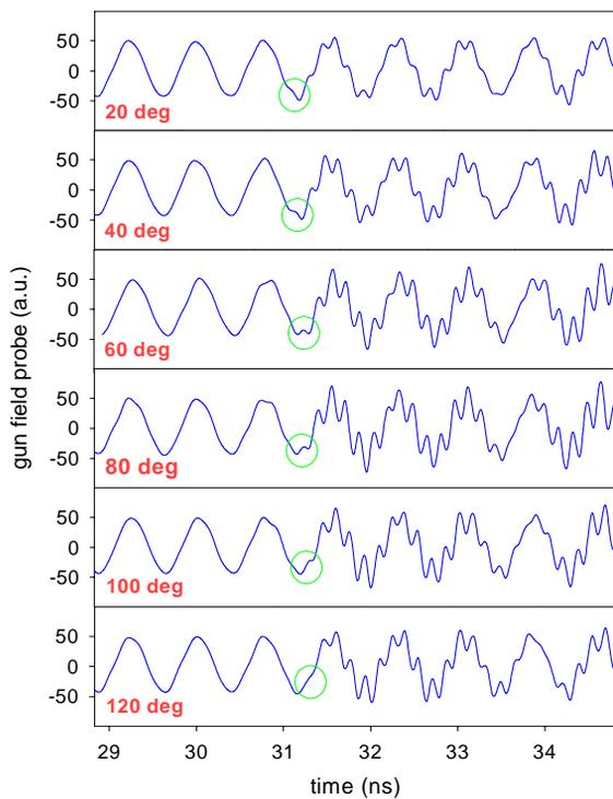
Figure 1: Gun field probe signals showing a couple of periods of the unperturbed 1.3 GHz RF field, followed by cycles that have the higher order mode perturbation superimposed on the fundamental mode. The small circles simply highlight the initial phase of the perturbation and its correlation with the electron beam launch phase (which is written next to each curve).
