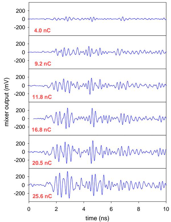
Figure 2: Output of RF mixer for various bunch charges.
