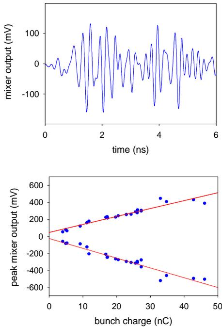
Figure 3: RF mixer output: (a) signal generated by a 43 nC electron bunch; (b) peak value of the wakefield amplitude plotted as a function of the charge in the drive bunch.
