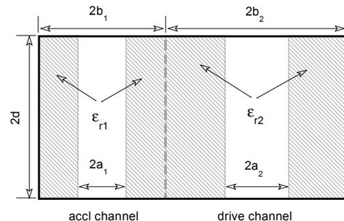
Figure 1: Dielectric two-beam WFA structure, with one vacuum channel for a decelerated (drive) beam and the other for an accelerated (test) beam.
