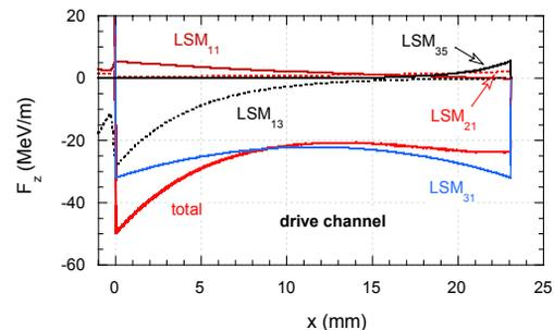
Figure 5: Axial wake field force  $F_z$ -profiles in acceleration and drive channels. Note scale difference.
