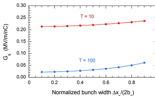
Figure 8: Dependence of gradient  $G_q$  on normalized bunch width  $\Delta x_b/(2b_2)$  for  $T = 10$  and  $T = 100$ , both with  $d = 20$  mm.
