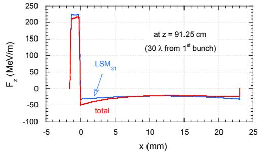
Figure 4: Axial wake field force  $F_z$  vs  $x$  for the design LSM<sub>31</sub> mode and for a superposition of 50 modes.
