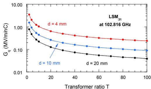
Figure 7: Dependence of gradient  $G_q$  in the acceleration channel produced by a unit charge in the drive channel on transformer ratio  $T$  for different half waveguide heights  $d$ .
