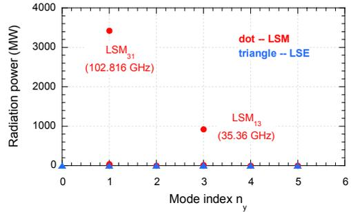
Figure 3: Mode radiation power spectrum, excited by a train of ten rectangular 500-MeV, 100-nC bunches with a spacing separation of  $L_b = 8.75$  mm.
