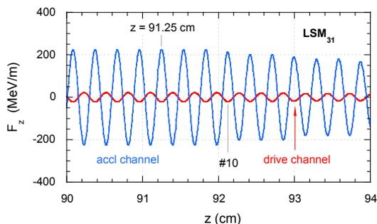
Figure 6: Axial wake field force  $F_z$  vs axial distance  $z$  in drive and acceleration channels for the design LSM<sub>31</sub> mode, when excited by ten 500-MeV, 100-nC bunches.
