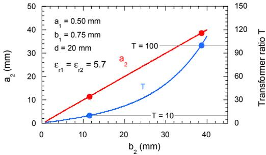
Figure 2: Dependence of drive beam channel half-width  $a_2$  and transformer ratio  $T$  on full drive channel half-width  $b_2$  for a 102.816-GHz two-beam WFA structure. Other parameters are as indicated in the figure.
