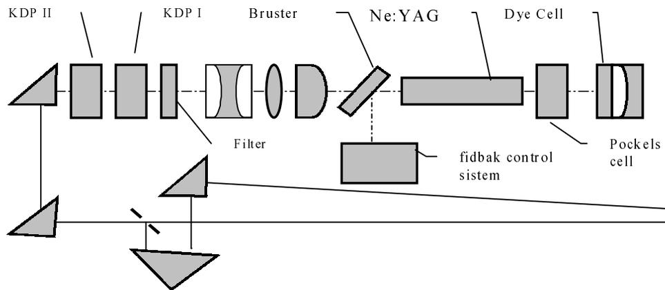
Figure 2: The scheme of laser set-up.
