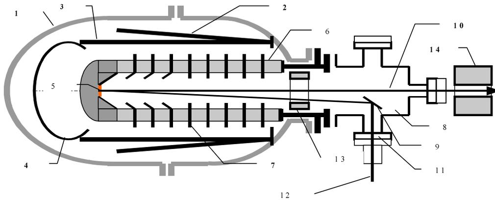
Figure 1: Schematic shape of the accelerator of electron bunches with photocathode. 1 - tank for gas, 2 - primary winding of the pulse transformer, 3 - secondary winding of the pulse transformer, 4 - high-voltage electrode, 5 - photocathode, 6 - isolation rings of accelerating tube, 7 - electrodes of accelerating tube, 8 - vacuum chamber, 9 - mirror, 10 - electron beam, 11 - vacuum tube, 12- laser beam. 13- magnetic focusing lens, 14 - electromagnetic focusing lens.
