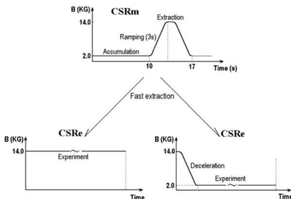
Figure 2: Magnetic field exciting procedure of CSR.
