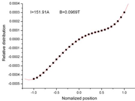
Figure 9: Dipole field distribution versus the radius.
