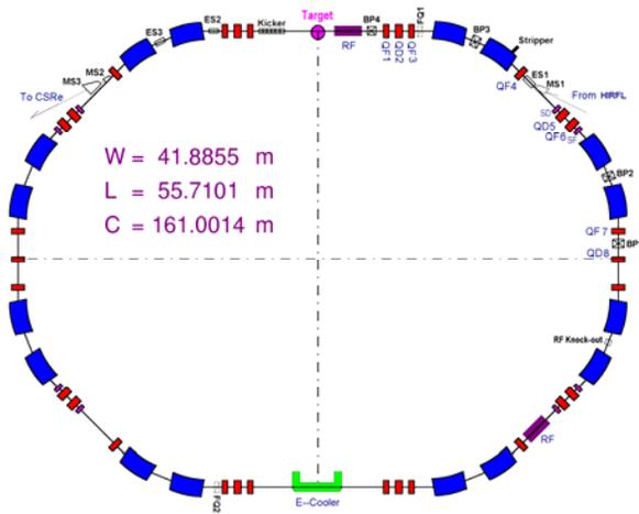
Figure 3: Lattice layout of CSRm.
