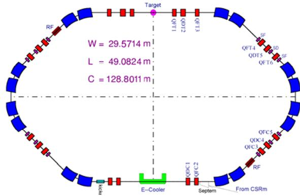
Figure 5: Lattice layout of CSRe.
