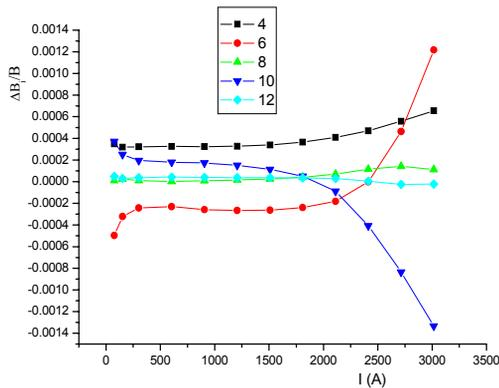
Figure 10: Multiple component errors in CSRm dipole.
