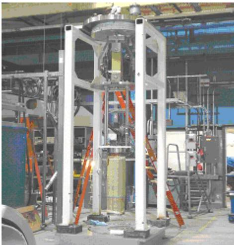
Figure 7: The superconducting insertion magnet coil #1 in the wiring stand.
