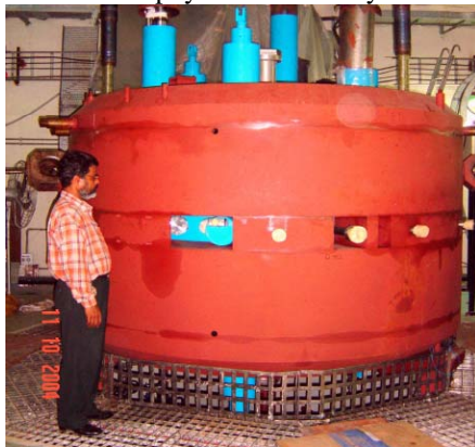
Figure 1: Cyclotron magnet with cryostat installed in it.
