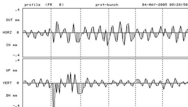
Figure 3: Horizontal (top) and vertical (bottom) orbit differences between two stores, measured at 150 GeV. Vertical scale is +/- 400 μm.
