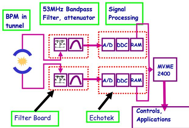
Figure 1: Tevatron BPM signal processing path
