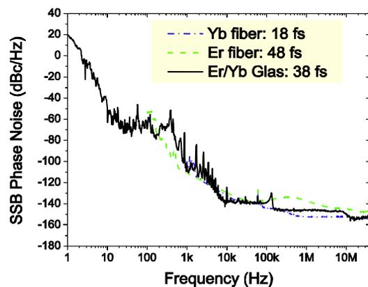
Fig. 7: Single-Sideband Phase Noise of an Yb-fiber laser, Er-fiber laser and Er/Yb-glass laser. The integrated timing jitter from 10kHz to 18MHz, i.e. half the repetition rate of the fiber lasers is stated explicitly.
