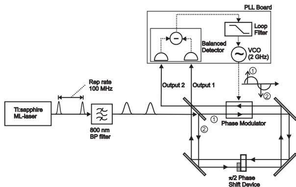
Fig. 4: Synchronization scheme for extraction of a 2 GHz signal from a 100 MHz repetition rate Ti:sapphire laser.
