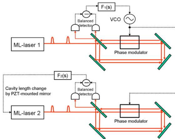
Fig. 8: Optical-to-optical synchronization scheme with the based on RF-synchronization techniques.
