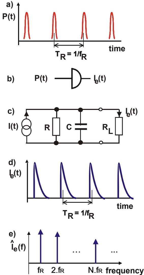
Fig. 2: a) Optical pulse train with instantaneous power  $P(t)$ ; b) Photo detection with external current  $I_e(t)$ ; c) Equivalent circuit of photo detector with external load; d) External current; e) Fourier components of external current.
