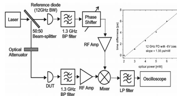
Fig. 3. AM-to-PM conversion factor measurement setup and the result when the reverse bias is set to 6 V. The measured slope is 1.56 ps/mW.
