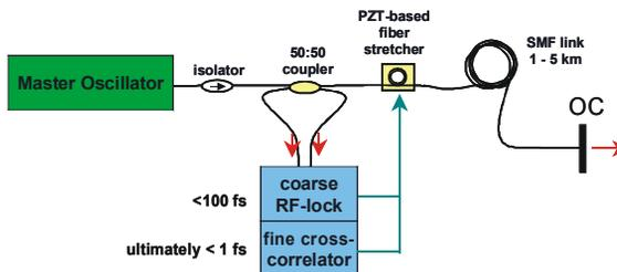
Fig. 5: Schematic of a timing stabilized fiber link. The coarse stabilization is accomplished by an RF-lock, whereas the fine adjustment will be accomplished by optical cross-correlation.
