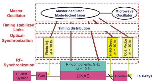
Fig. 1: Schematic outline of timing distribution and synchronization for FEL facility.
