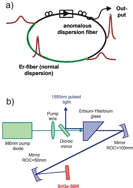
Fig. 6: Schematic of (a) a stretched pulse Er-fiber laser mode-locked by nonlinear polarization rotation and (b) an Er/Yb-glass laser mode-locked by a semiconductor saturable absorber mirror.
