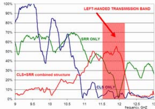
Figure 7. Amplitude of the transmission through SRR-only, CLS-only and combined structures on a linear scale. Red zone is a left-handed transmission band, the frequency range, where SRR-only and CLS-only metamaterials do not exhibit transmission (~5%), but combined structure provides almost 50% power transmission – signature of left-handed metamaterial.
