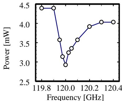
Figure 4: Power measured by the diode attached to frequency meter. Dip at 120.0 ± .025 GHz consistent with
