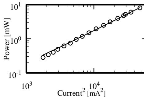
Figure 3: CTR power measured by the diode as a function of the beam current squared. Solid lines is linear fit to circular data points.
