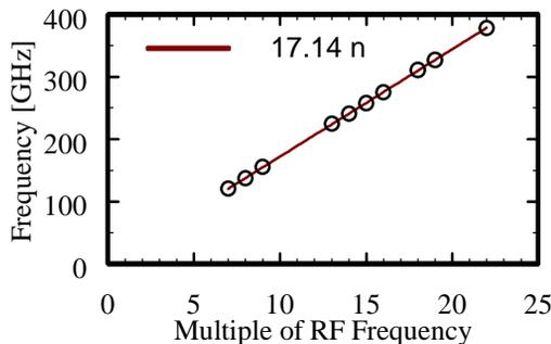
Figure 5: CTR Spectrum measured with double heterodyne receiver, plotted against the multiple of the RF frequency of 17.14 GHz.
