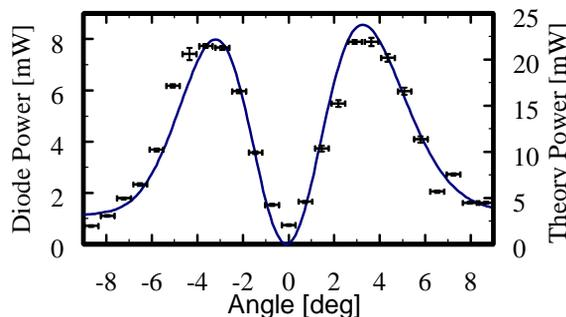
Figure 2: Angular distribution of CTR power measured by the diode, points, and theory calculations made with EFIE code, shown by the blue line.
