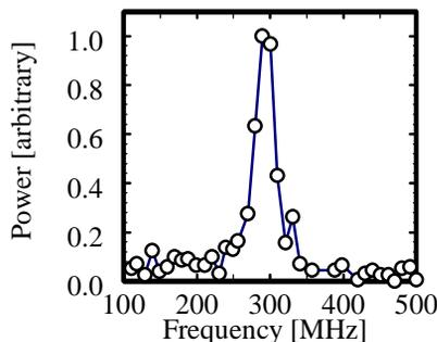
Figure 6: FFT at 240 GHz showing 28 MHz FWHM.
