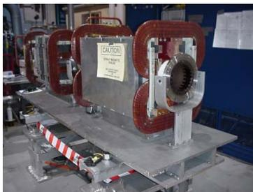
Figure 8: Long Injection dynamic bum magnets with Beam Pipe and Bellow.
