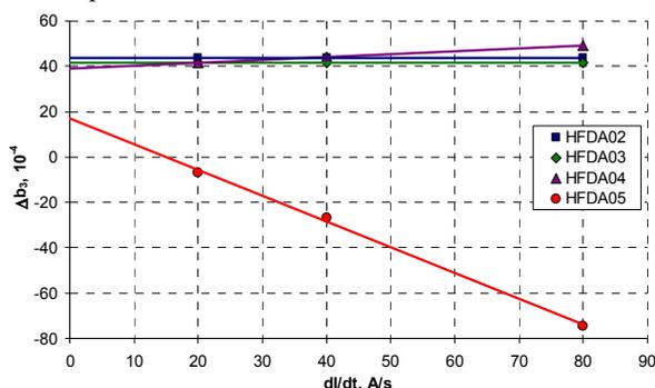
Figure 6: Sextupole loop width at bore field  $B_0 = 2$  T.
