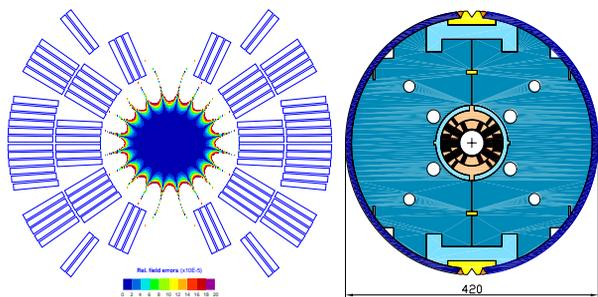
Figure 1: HFDA coil and magnet cross-sections.
