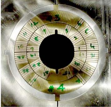
Figure 3: HFDA02 coil cross-section.
