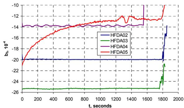
Figure 7: Sextupole decay at  $I = 3$  kA (HFDA02-04) and  $I = 2.4$  kA (HFDA05).
