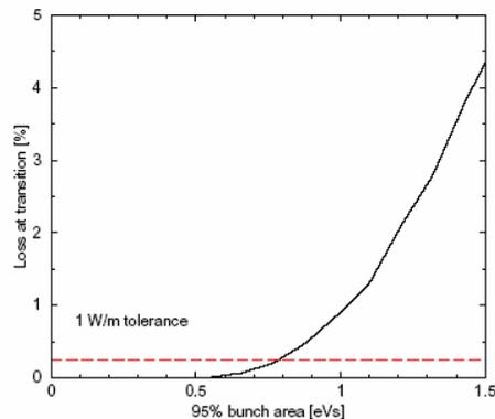
Figure 3: Expected fractional beam loss during transition as a function of the initial (95%) longitudinal beam area obtain with computer code TIBETAN.
