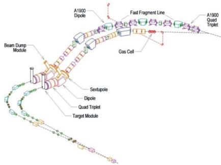
Figure 1: Possible layout of RIA's fragment separators. Magnets downstream of the pre-separator may be like those in the NSCL's A1900 FRS. Horizontal layouts are also being considered.
