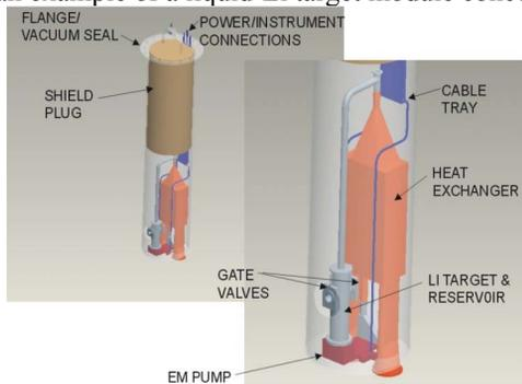
Figure 2: Conceptual design of a target module for an electromagnetically-pumped liquid-lithium target.
