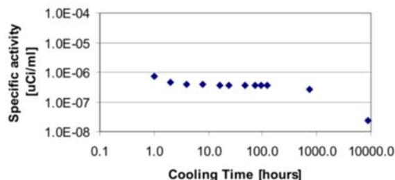
Figure 4: Residual activity in air region above the module as a function of cooling time.
