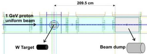
Figure 5: Configuration used in MARS15 for ISOL beam dump calculations.
