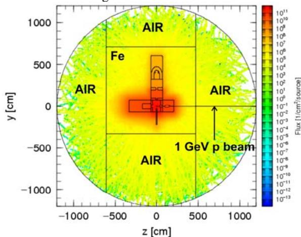
Figure 2: Top view of the ISOL module in PHITS and calculated neutron flux in the system.
