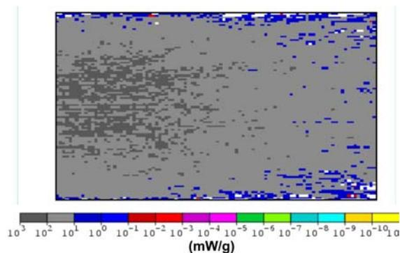
Figure 7: Heat deposition in the ISOL beam dump. The beam dump material is a mixture of 90% graphite and 10% water.
