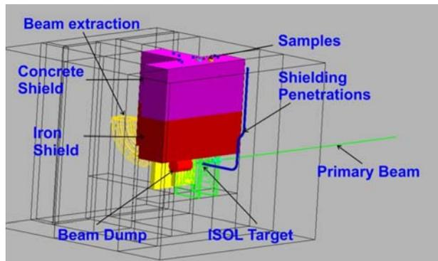
Figure 1: ISOL module geometry used in simulations. The steel shielding is shown as wire-frame.
