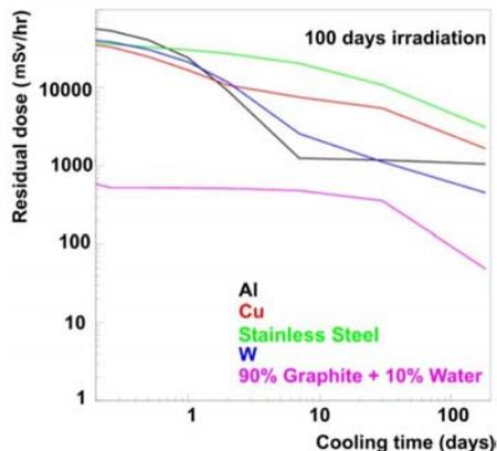
Figure 6: Residual dose at contact for different beam dump materials.
