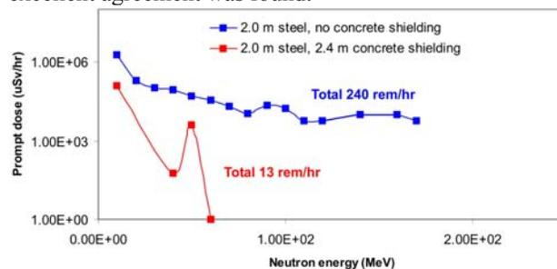
Figure 3: Prompt dose due to neutrons in the air region above the ISOL module.
