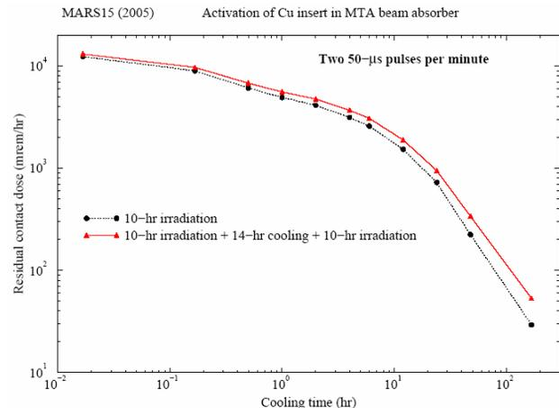
Figure 3. Residual activation of Cu insert in beam absorber. (Two 50- $\mu$ s pulses provide  $4.3 \times 10^{11}$  p/sec.)
