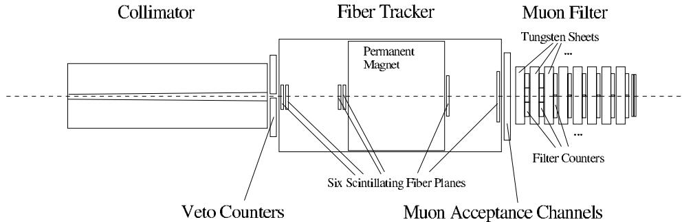
Figure 2: Schematic Drawing (top view) of the LMC.
