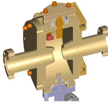
Figure 2: 1.3 GHz ELBE-style buncher cavity.
