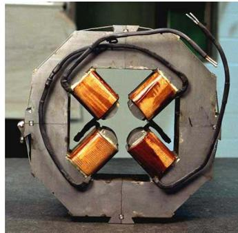
Figure 3: Fermilab 5cm long, 5cm bore quadrupole.
