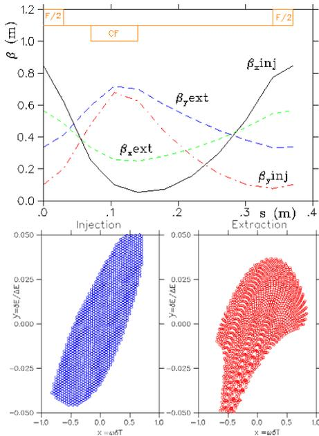
Figure 1: Lattice functions and longitudinal phase space plots for 10-20 MeV electron model.
