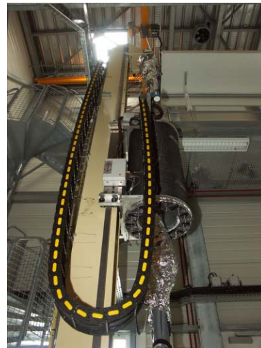
Fig. 2 Wiggler vacuum chamber during NEG deposition at ESRF.
