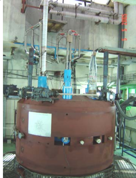
Figure 1: Cyclotron magnet assembly with cryogenic systems.
