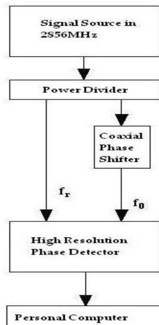
Figure 2: Configuration of precise phase detector.
