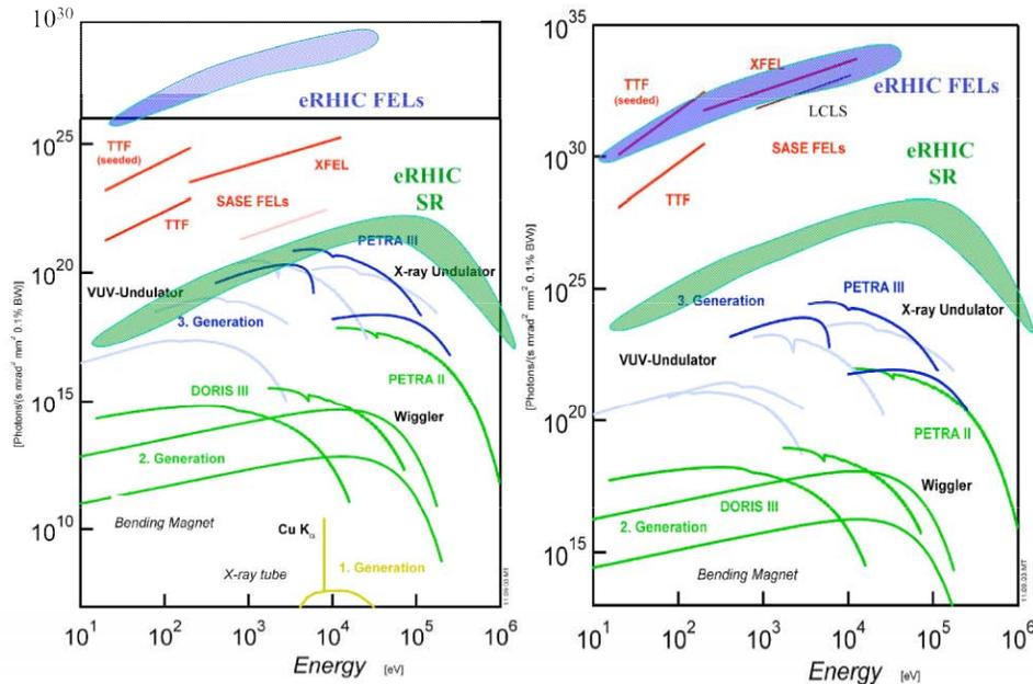
Fig.3 Average and peak spectral brightness of eRHIC light source (blue – FELs, green – spontaneous radiation) compared with other sources. While being similar to SASE FEL sources in peak spectral brightness, the average spectral brightness of eRHIC FELs would exceed the rest of the light sources (existing and proposed) by about 5 orders of magnitude.
