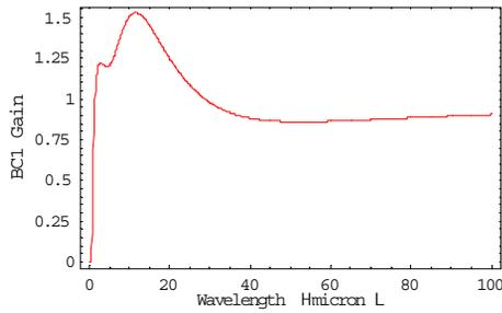
Figure 2: Gain of density modulation at exit of BC1.
