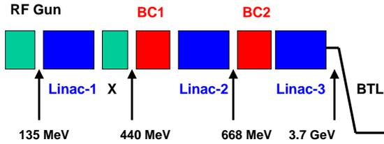
Figure 1: Layout of the PAL-XFEL accelerator system.
