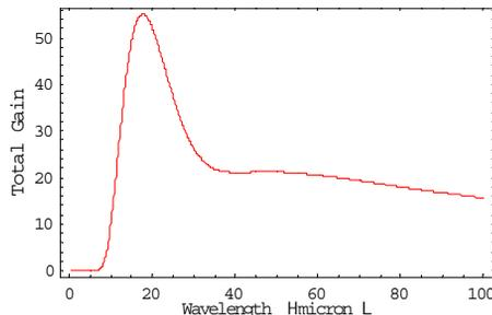
Figure 7: Total gain of the density modulation due to the LSC wake and the linac wake at the exit of BC2.
