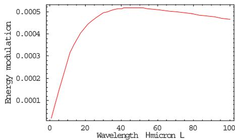
Figure 3: Gain of energy modulation at the exit of BC1.
