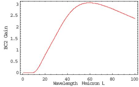
Figure 4: Gain of density modulation at the exit of BC2.
