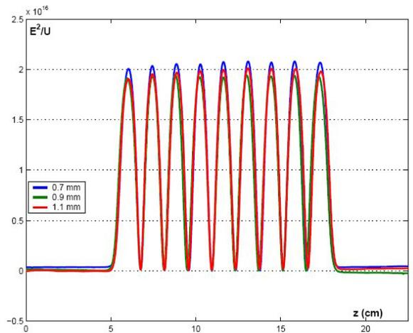
Figure 8: measured longitudinal electric field on axis.
