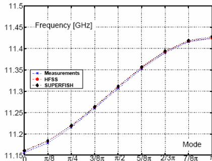
Figure 7: measured dispersion curve.
