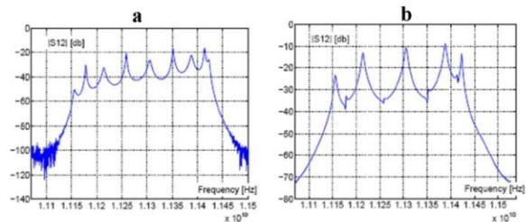
Figure 5: transmission coefficients between the two small antennas and coupler input port.
