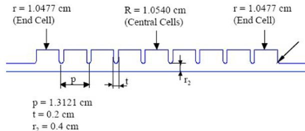
Figure 2: 2D profile of the X-band structure.
