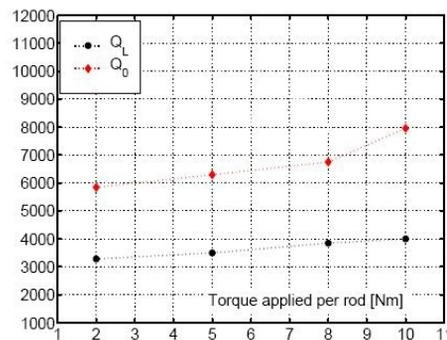
Figure 6: measured quality factor of the  $\pi$  mode resonance as a function of pressure realized by the rods.
