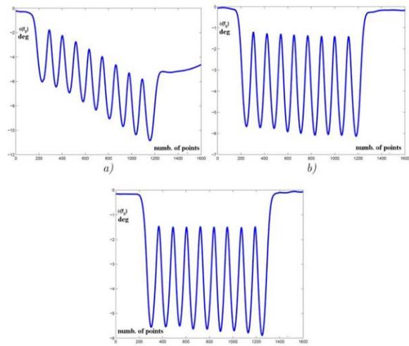
Figure 8: phase of resonance measurement with different wire diameters: a) 0.18 mm; b) 0.148 mm; c) 0.083 mm.
