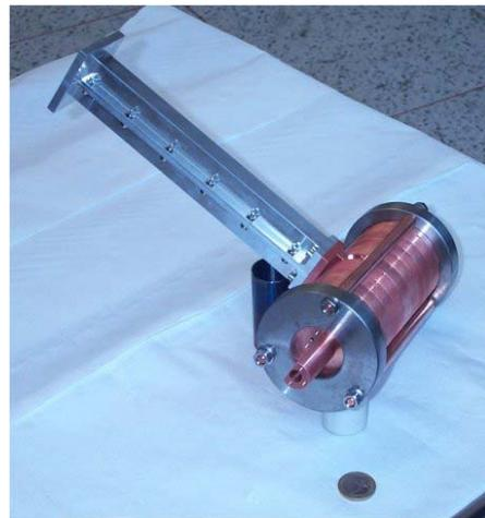
Figure 4: copper prototype of the X band structure.
