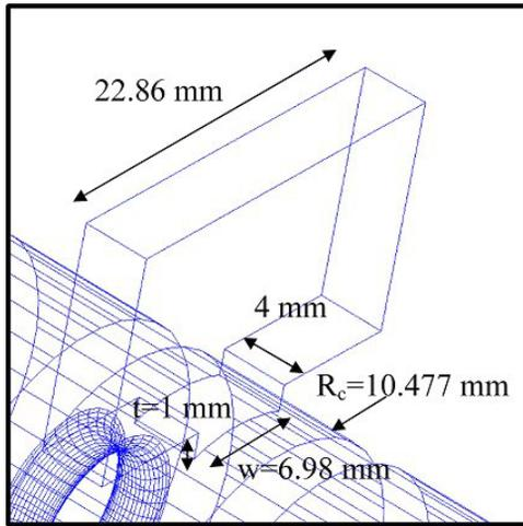
Figure 3: sketch of the coupling cell.
