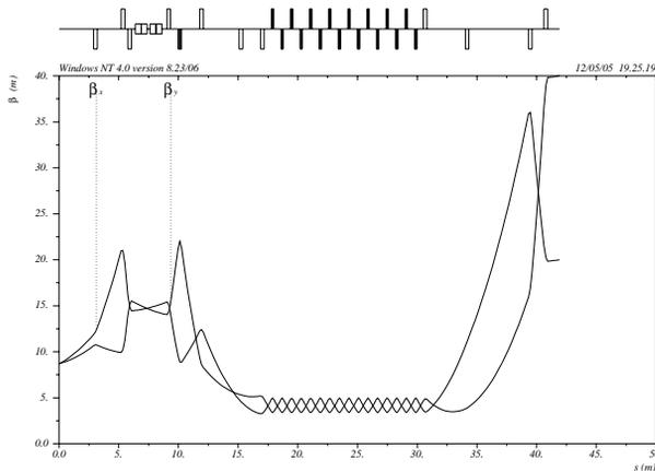
Figure 2: Evolution of the  $\beta$ -functions in the diagnostic section 1.
