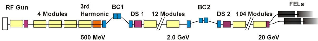
Figure 1: Accelerator layout of the European XFEL Project (BC: bunch compressor; DS: diagnostic section).
