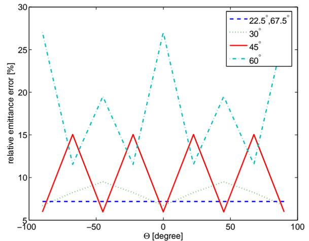
Figure 4: Resulting emittance errors as a function of  $\Theta$  for  $M = 4$ , a beam size error of 10% and total of 16 beam size measurements for all lattices.
