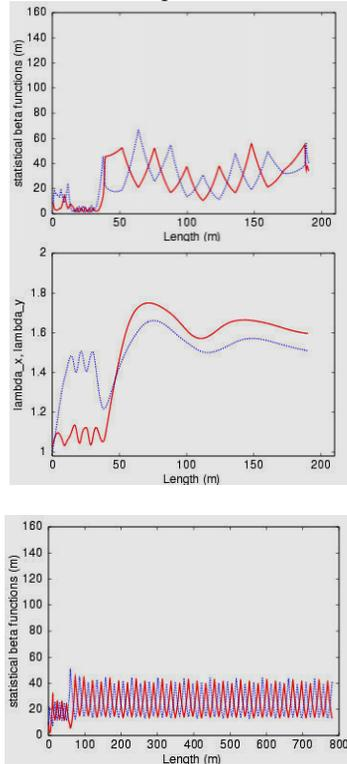
Figure 2: Space charge effects of 1 kA peak current on optics downstream of compressor chicane. Upper two pictures: optics and mismatch parameter downstream of 1<sup>st</sup> chicane (1 kA peak current, 500 MeV beam energy). Lower Picture: No effect downstream of 2<sup>nd</sup> chicane (5 kA peak current at 2.5 GeV). The red curves show parameters in the horizontal plane, the blue one in the vertical.
