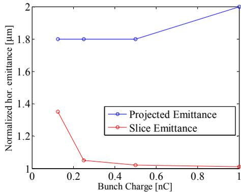
Figure 5: Normalized horizontal emittance after 2<sup>nd</sup> chicane vs. bunch charge for fixed peak current of 5 kA.
