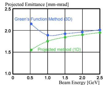
Figure 3: Projected emittance vs. beam energy (Strength of 2<sup>nd</sup> chicane bending magnets scales with energy).
