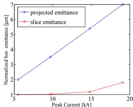
Figure 4: Normalized horizontal emittance vs. different peak currents due to different settings of the 2<sup>nd</sup> bunch compression chicane.
