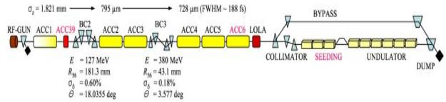
Figure 1: TTF2 layout for the fs FEL mode.
