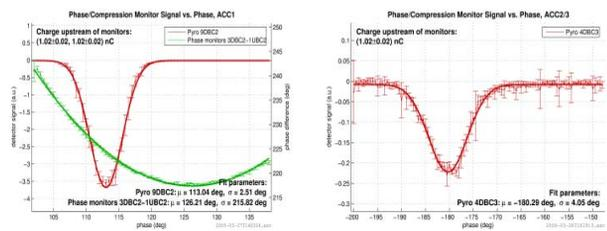
Figure 6: Measured pyroelectric detector and phase monitor signals: (left) at 9DBC2 while ACC1 phase is scanned and (right) at 4DBC3 while ACC2 and ACC3 phases are simultaneously scanned under on crest ACC1 phase.
