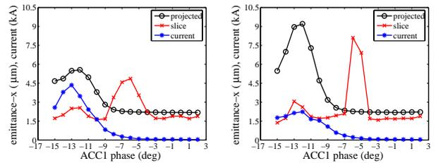
Figure 5: Simulation results on projected and slice normalized rms horizontal emittances and peak current after BC2 (left) and after BC3 (right).
