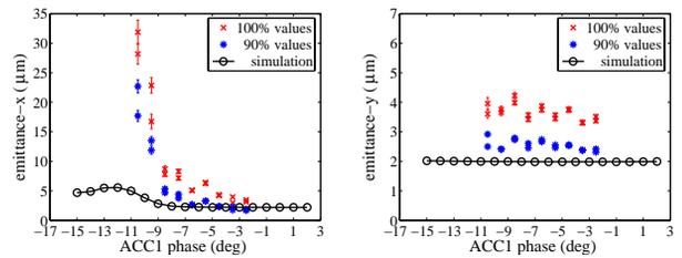
Figure 4: Simulation and measured results on projected emittance after BC2 for different ACC1 phase: (left) projected normalized rms horizontal emittance and (right) projected normalized rms vertical emittance.
