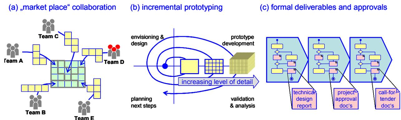
Figure 1: Boundary conditions on collaborative planning procedures: (a) groups self-organize into expert teams for specific tasks, introducing the need for coordination; (b) planning benefits from prototypes which are analyzed and iteratively and incrementally detailed; (c) authorities expect pre-defined deliverables for project approvals.
