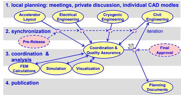
Figure 4: Planning process for the XFEL.
