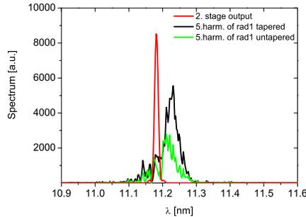
Figure 4: Spectral power distributions of the fifth harmonic of the first radiator and of the fundamental of the second radiator are shown. The spectral distribution of the fifth harmonic is depicted for the tapered and untapered case.
