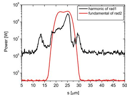
Figure 3: Comparison of the power distributions of the second radiator and the fifth harmonic of the first radiator after the tapered section.
