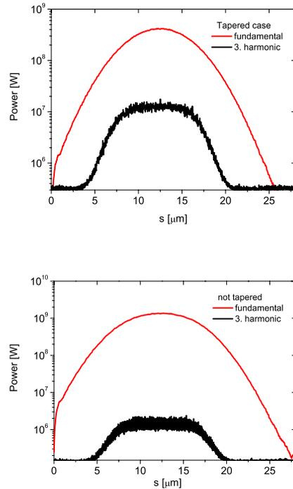
Figure 2: The power distribution of the third harmonic and of the fundamental at the saturation point of the third harmonic. The power distributions for the tapered (top) and untapered (bottom) case are depicted.
