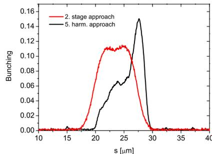
Figure 5: Comparison of the bunching factors achieved by the harmonic radiation and the second radiator output.
