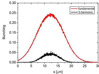
Figure 1: Comparison of the bunching factors of the fundamental and third harmonic for the final amplifier of HE-FEL after 7.13 m. Bunching along the electron beam is shown.
