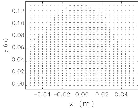
Figure 4: Dynamic aperture for optimized abstract lattice (the window size is  $\pm 20 \times 20 \sigma_{inj}$ ).
