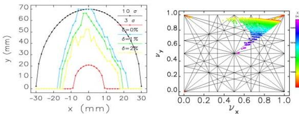
Figure 7: Dynamic aperture and tune footprint for the optimized lattice.
