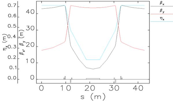
Figure 2: Optical functions of normal TME cell ( $150^\circ$ ).
