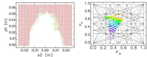
Figure 1: Dynamic aperture and footprint of original design (aperture scale is  $\pm 10 \times 10$  sigma of injected beam).
