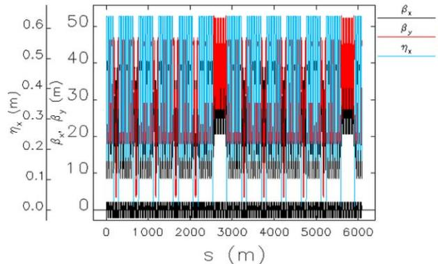
Figure 5: Optical functions of 6-km ILC damping ring.
