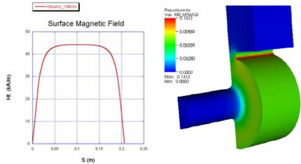
Figure 7: RF pulse heating calculations.
