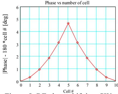
Figure 5: RF phase shift in a SW structure.
