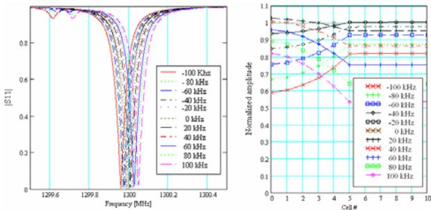
Figure 6: Frequency spectrum (left) and electrical field amplitude (right) for various frequency changes.
