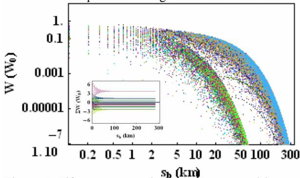
Figure 5: Fifty separate wakefields (represented by each separate color) at the location of each bunch (2820 are shown). The wake is normalized with respect to  $W_0 = 0.11$  V/pC/mm/m. Also shown inset, is the sum wakefield for each of the 50 wakefields.
