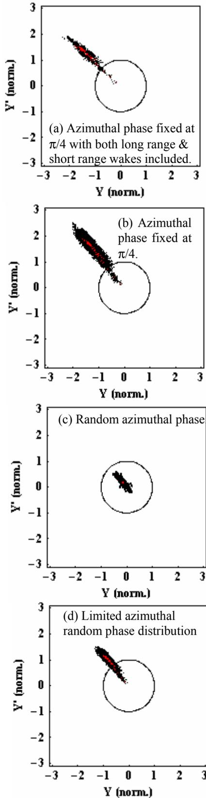
Figure 2: Phase space at end of linac. In (a) 16 machines are simulated. The results of tracking 500 bunches down 200 machines under the influence of *long range wakes* only are illustrated in (b) through (d) for several different azimuthal angle distributions.
