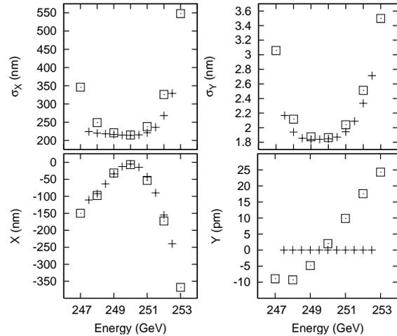
Figure 4: Impact of NLC BDS nonlinearities on off-energy beam parameters. Cross = Bmad, Box = LIAR/DIMAD.
