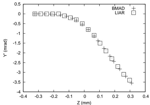
Figure 1: Macroparticle deflection along a bunch resulting from an offset NLC cavity with transverse wakefields.
