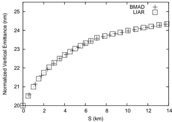
Figure 3: Vertical normalized emittance growth in the TESLA main linac resulting from an initial vertical beam offset equal to the injected beam size.
