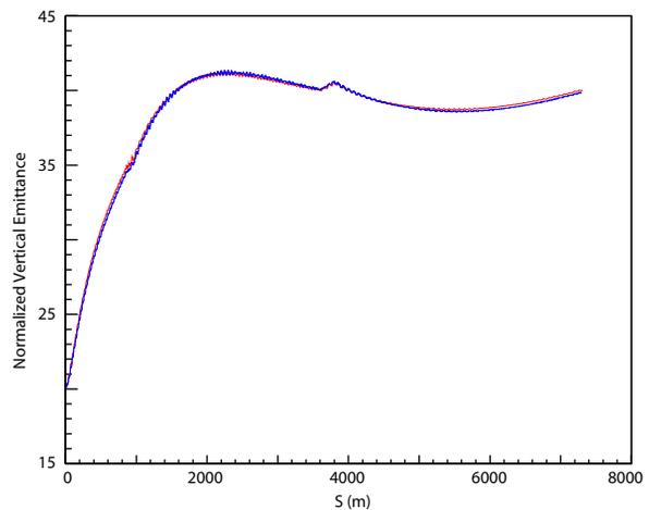
Figure 2: Vertical normalized emittance growth in the NLC main linac resulting from an initial vertical beam offset equal to the injected beam size.
