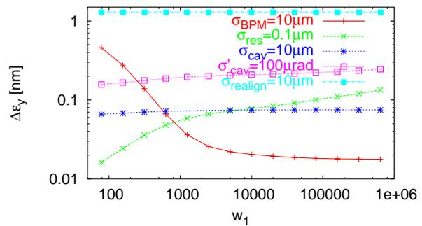
Figure 2: The final beam emittance growth as a function of the weight  $w_1$  for the different error sources separately.
