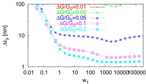
Figure 1: The final beam emittance as a function of the weight  $w_1$  for the trajectory differences for different gradient variations.
