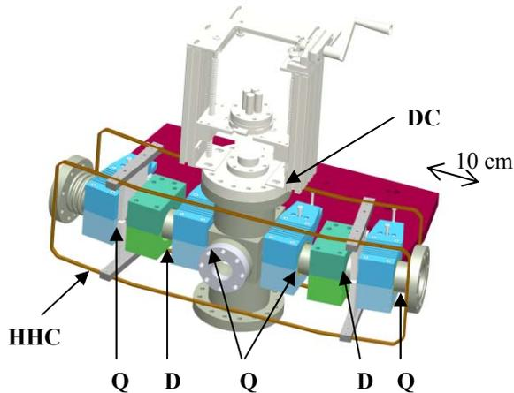
Figure 3: A scaled drawing of a UMER ring section, showing the locations of dipoles (D), quadrupoles (Q), Helmholtz coils (HHC) and the diagnostic chamber (DC).
