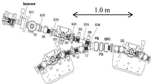
Figure 2: A scaled drawing of the UMER matching beam line, Y-Section and two ring sections showing magnet placement. Labels are explained in the text.
