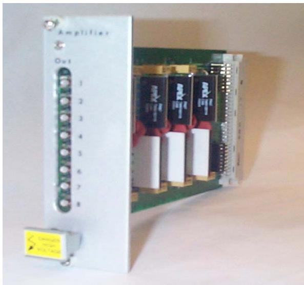
Figure 3: Deflection plates high-voltage amplifier.
