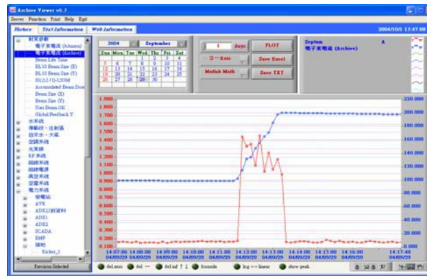
Figure 5: The beam current and the leakage current of septum while beam injection on. (2004/09/29 PM2:11~2:14)
