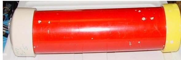
Figure 1B: 1-Foot Detector in ABS Housing.
