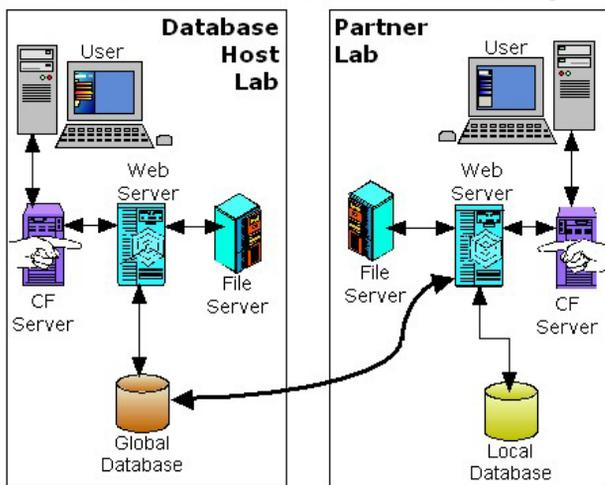
Figure 3: Architecture for accessing central database from remote partner sites using local interface programs and analysis tools.
