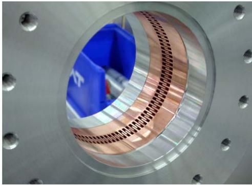
Figure 4: Comb-type RF shield for gate valve.
