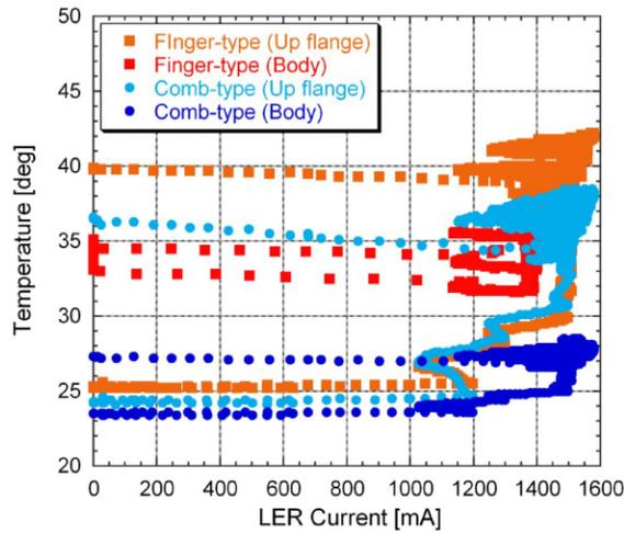
Figure 5: Temperatures at connection flange and body of gate valves with comb-type and finger-type RF shield. The data include those during several beam injection cycles. Small decreases of temperatures at low beam currents are due to the large heat capacity of gate valve.
