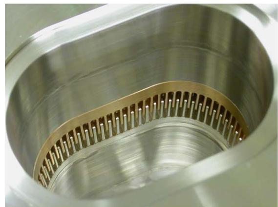
Figure 1: Racetrack bellows chamber with comb-type RF shield.
