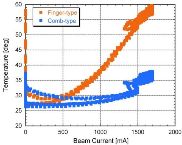
Figure 2: Average temperatures of corrugations of four bellows with comb-type and finger-type RF shield. The data include those during several beam injection cycles.
