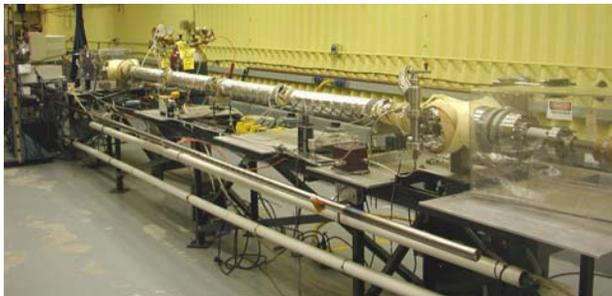
Figure 4: Magnetron sputtering set-up for NEG coating of 4.0m long x 7.6cm ID RHIC experimental beryllium beam tubes. Shown is the stainless steel test beamtube with distributed viewports.
