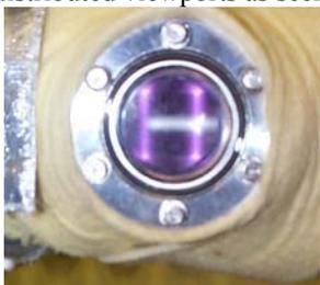
Figure 9: Typical discharge observed at all viewports of test beam tube using the 1" diameter supported cathode.
