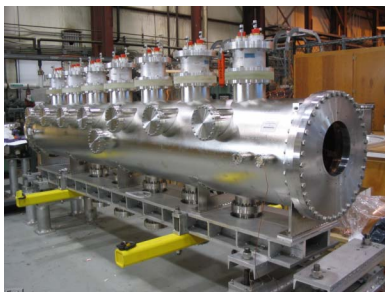
Figure 7: Seven extraction kicker magnets assembled inside one large vacuum chamber.
