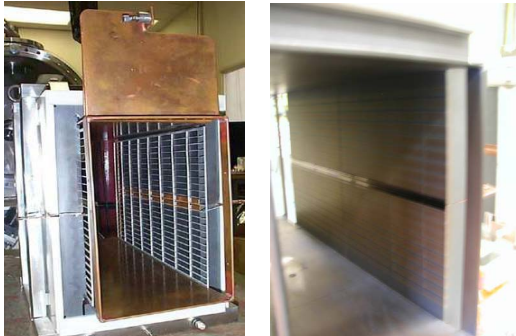
Figure 6: The extraction kicker module with coating masks (left) and with coated TiN strips (right).
