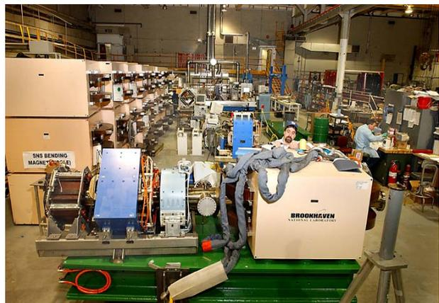
Figure 1: Typical Half-cell assembly with vacuum chamber.
