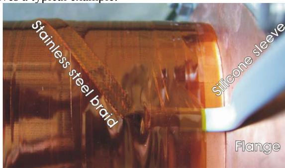
Figure 3: Electrical connection of heater bands.
