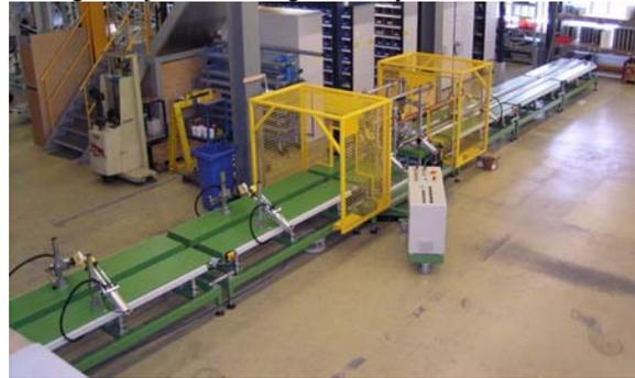
Figure 7: Wrapping machine; insertion table left, wrapping unit middle, traction unit right
